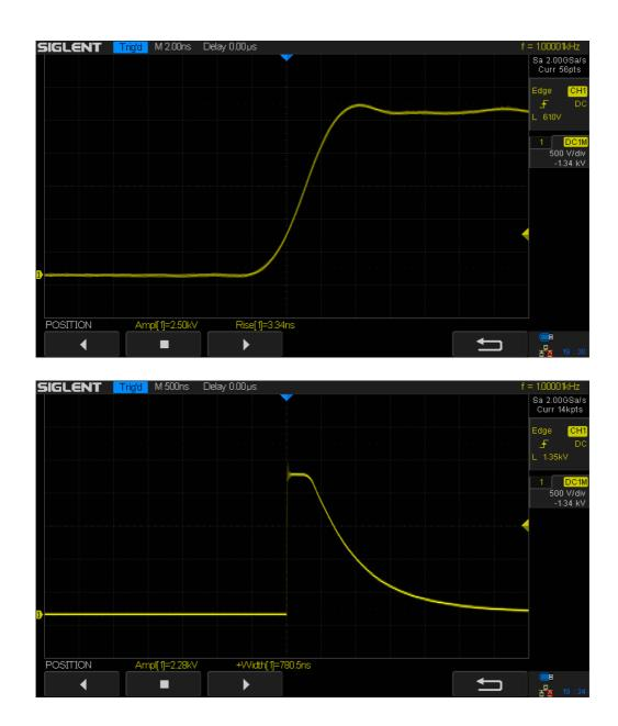
Typical Electrical Responses Measured with 1m  $50\Omega$  Cable
